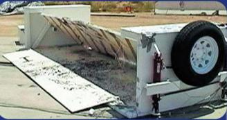
**MP5000** – A mobile, crash barrier can be towed into position by a medium-sized pick-up truck or equivalent and deploy in 15 minutes to stop & disable a 15,000 lb (66.7 kN) G.V.W. vehicle moving at 40 mph (64 kph).
